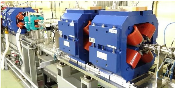
Figure 2: Photo of the new pulsed Q magnet.
