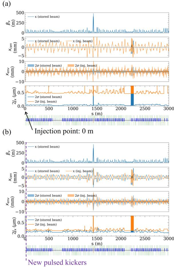
Figure 4: Comparison of (a) present betatron injection and (b) AS injection schemes, with stored (blue) and injected (orange) beams after the injection. The graph shows, from top to bottom, the horizontal beta function of HER optics, beam orbits,  $2\sigma$  beam envelopes, and actions  $2J_x$ .
