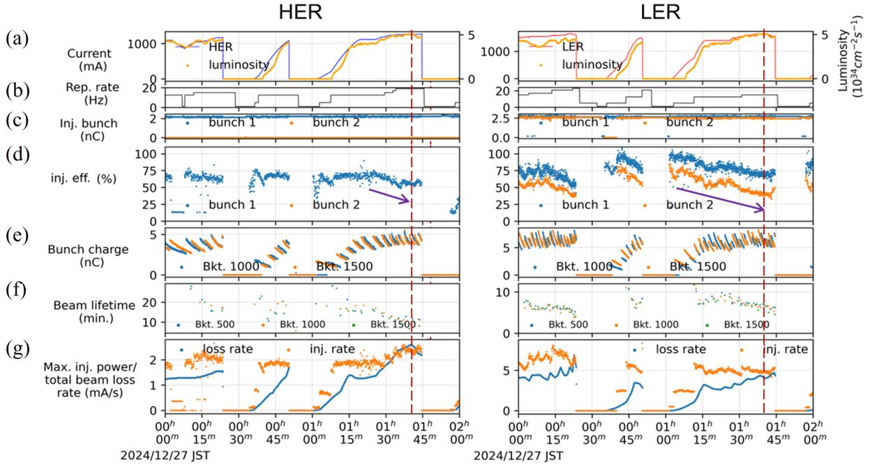
Figure 2: Injection overview of HER (left) and LER (right): (a) storage currents and luminosity, (b) injection frequencies, (c) bunch charges at the injector ends, (d) injection efficiencies, (e) bunch charges and (f) beam lifetimes at some buckets, and (g) injection powers and beam losses. The dashed red lines correspond to the peak luminosity.
