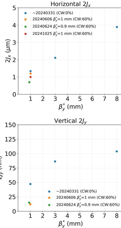
Figure 1: Measured horizontal (top) and vertical (bottom) dynamic apertures of HER with different  $\beta_y^*$  values and crab waist (CW) conditions.
