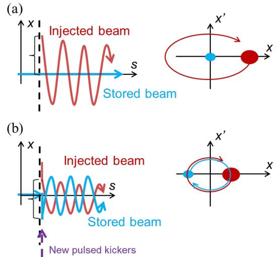
Figure 3: Schematic comparison of the two injection schemes: (a) conventional betatron and (b) aperture sharing (AS) injections. The stored (blue) and injected (red) beams around the injection are illustrated.
