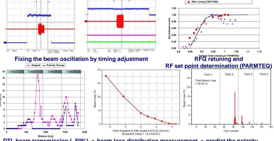
DTL beam transmission (~50%) -> beam loss distribution measurement -> predict the polarity mistake of QM by using PARMILA -> QM polarity reversal ->beam transmission (100%)
