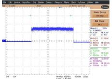
Long pulse operation (LEBT beam, 2ms pulse)
