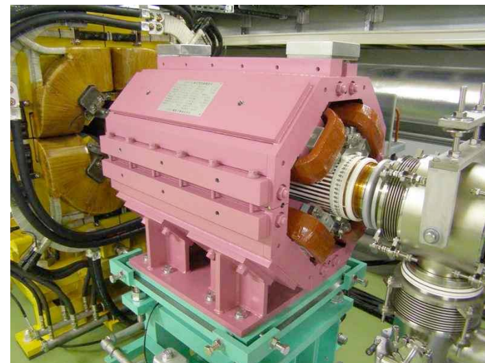
RQ: for ripple compensation ( < 3 kHz)
