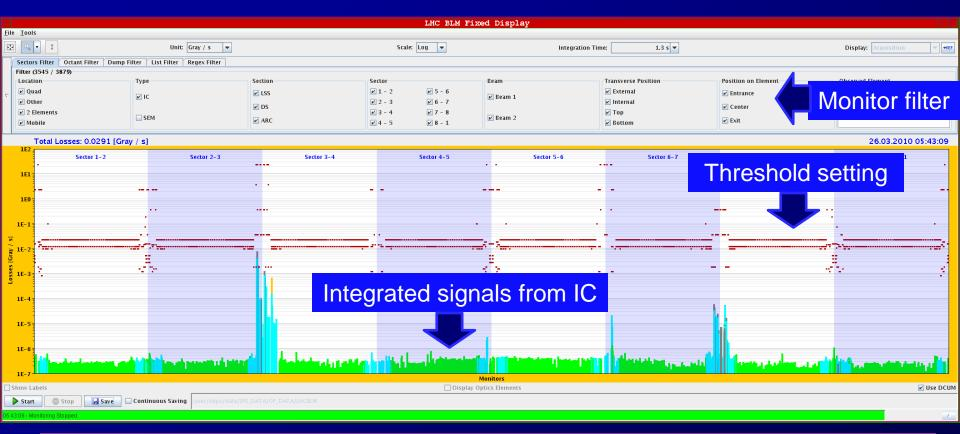
Beam loss monitor readings (Gray/s) along the ring (integration time : 1.3 s) Updating @ 1Hz Losses units: Gray/s, % or normalized Linear or logarithmic scale
