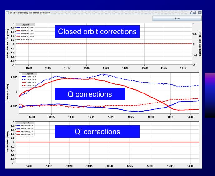
Q – feedback is now routinely in use during ramps (not yet with PLL)
