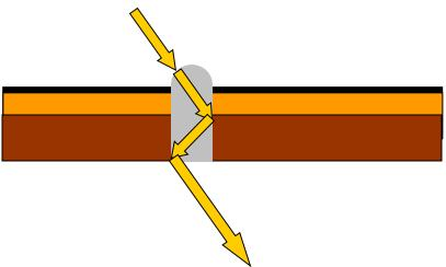
A metallized tube reflects daylight into the room.
