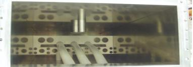
Leak from the RF load cooling line joint
