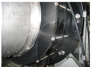
Water leakage at klystron oil tank
