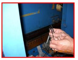
• The new O-Ring was greased and installed.
