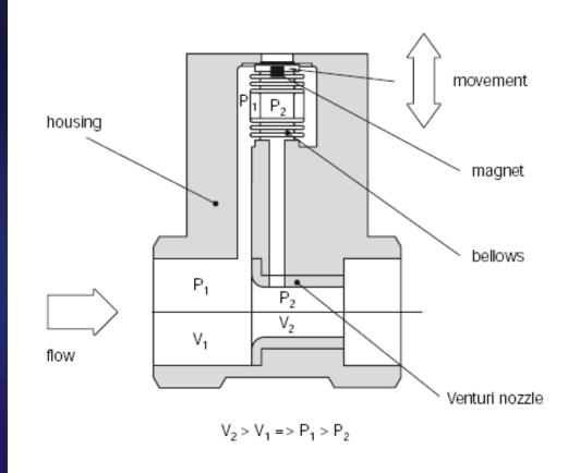
Stainless Steel construction, no moving parts, remote digital readout Differential Pressure with Hall effect monitor
