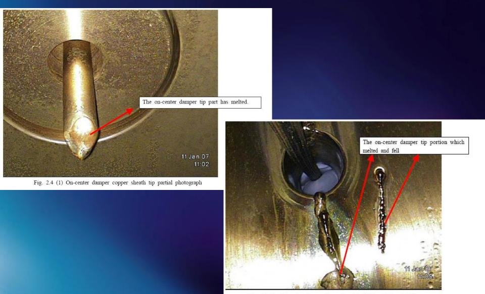
Fig. 2.4 (3) On-center damper tip portion (2) which melted and fell
