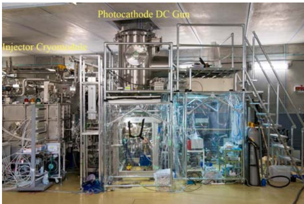
Figure 4: Injector of the Compact ERL including the photocathode DC gun and an injector cryomodule.
