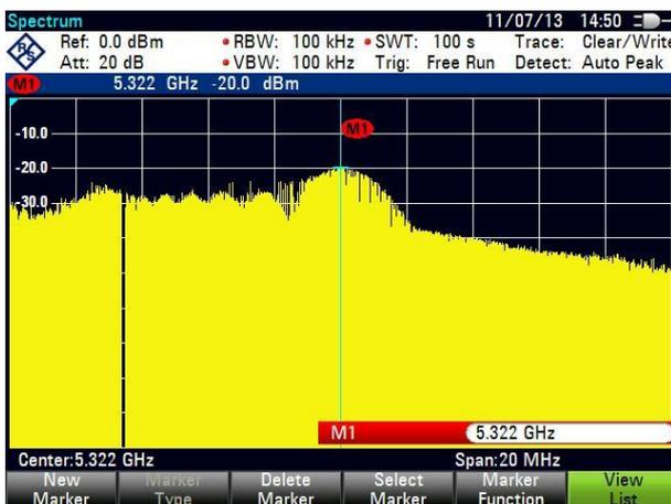
Figure 10: Frequency spectrum generated from the magnetron.
