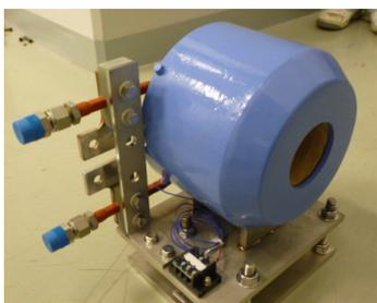
Figure 2: Water-cooled solenoid coil for LEENA.
