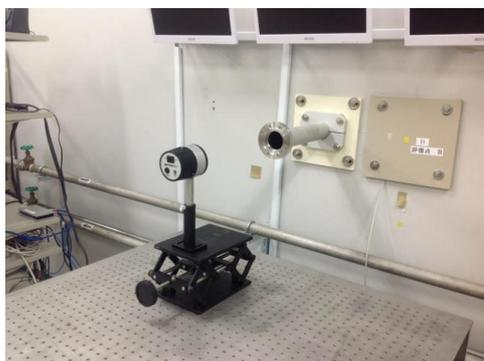
Figure 7: THz beamline and optical bench in the user experimental room.
