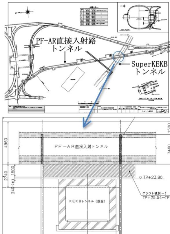
Figure 4: New beam transport line for PF-AR.
