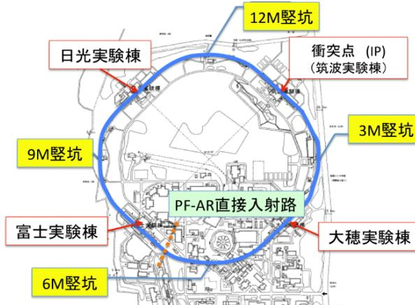
Figure 1 : SuperKEKB main ring indicated in blue and the construction sites on the ground surface.
