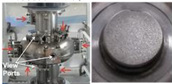
Figure 3: Photo of 1-cell coupon cavity(left) and φ 8mm coupon(Right).
