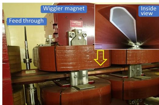
Figure 9: Beam pipe with clearing electrode inside for LER wiggler magnets.
