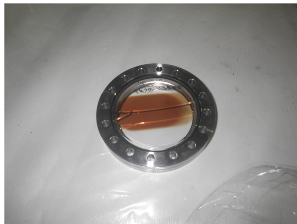
Figure 4: Cracked viewing port.
