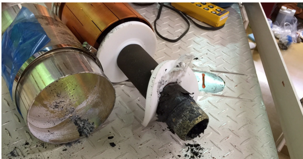
Figure 5: Damaged coaxial tube and teflon plates.
