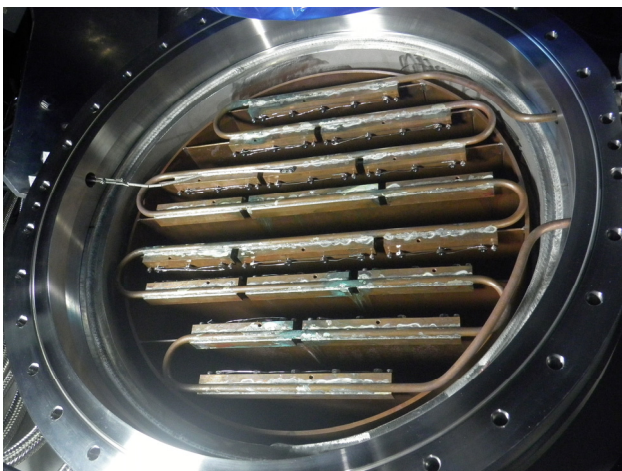
Figure 6: Cooling baffles coated with patina.
