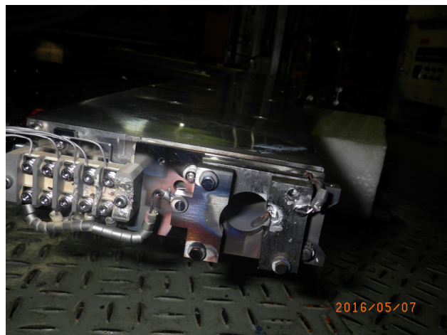
Figure 3: Picture of MDC1 for RRC. Bolt that secure the baffle plates was melted.
