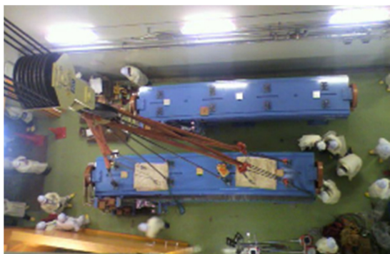
Figure 5: Photo of a failed BM#67 (top) and a reference BM (bottom).
