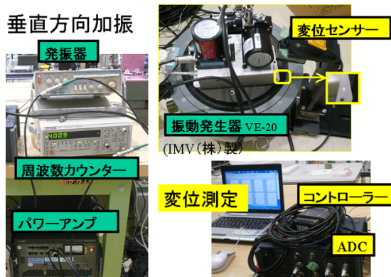
Figure 8: Oscillation arrange for frequency characteristics measurement of vertical direction.
