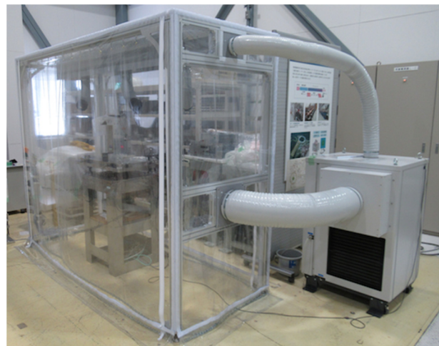
Figure 6: Temperature controlled booth for temperature coefficient measurement of permanent magnet circuit.
