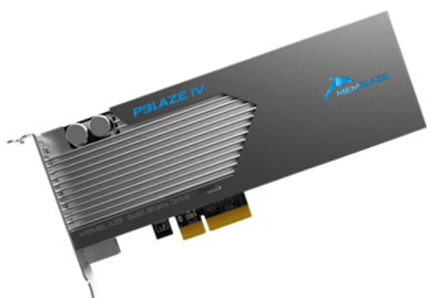
Figure 1: Photograph of PBlaze4 that is installed as main storage on RIBFCAS slave server.
