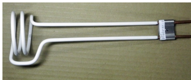
Figure 6: Photograph of a J-PARC antenna.
