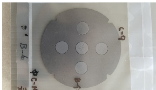
Figure 8: A picture of a graphite filler and five specimens of SiC coated graphite, which are included in an irradiation capsule. The graphite with a diameter of 10 mm and a thickness of 0.8 mm is coated by CVD-SiC with a thickness of 0.1 mm. Several sorts of graphite are installed for comparison.
