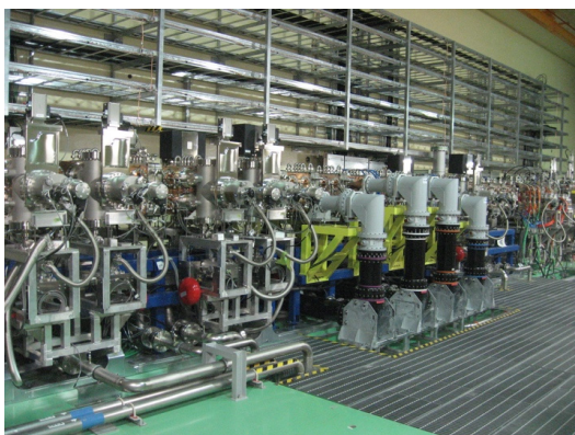
Figure 7: RF conditioning of RFQ.
