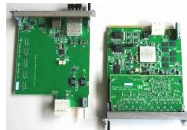
Figure 7: LLRF control board MTCA.4 are connected by optical link to make vector sum calculation digitally for 8 cavities pickup signals.
