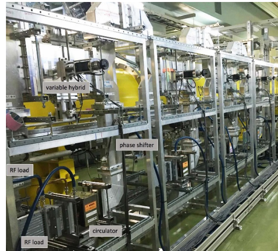
Figure 6: Realized RF power distribution scheme of STF phase-2 cryomodule. The waveguide components are built in the support frame.
