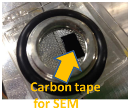
Figure 11: Conductive carbon tape prepared at the top of a rough pumping system to collect the dust during the evacuation.
