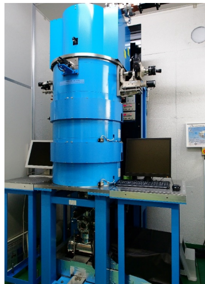
Figure 1: The prototype relativistic ultrafast electron microscopy using a photocathode rf gun.
