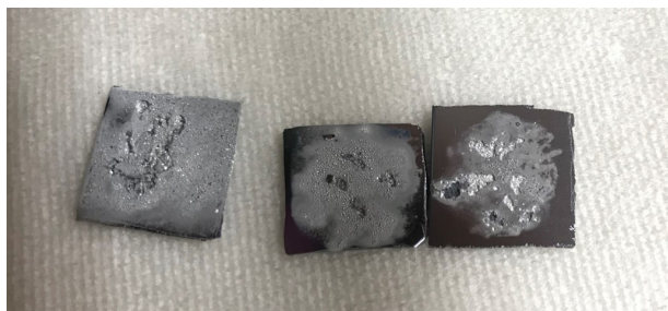
Figure 4: The Si substrate after heat cleaning at a higher temperature than 900°C.
