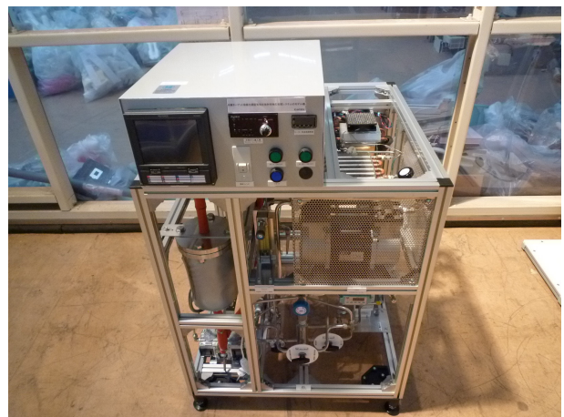
Figure 5: New testing instrument for gaseous elements trap system.
