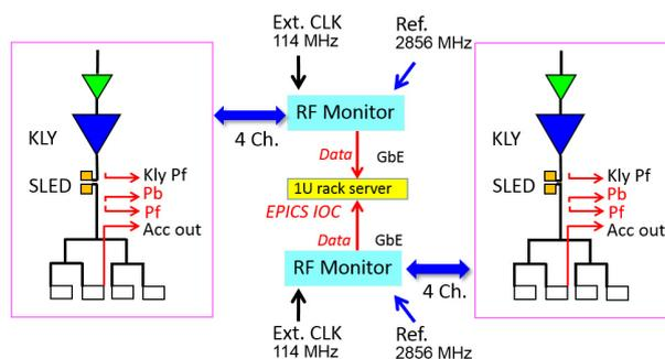
Figure 1: Block diagram of RF monitor system.
