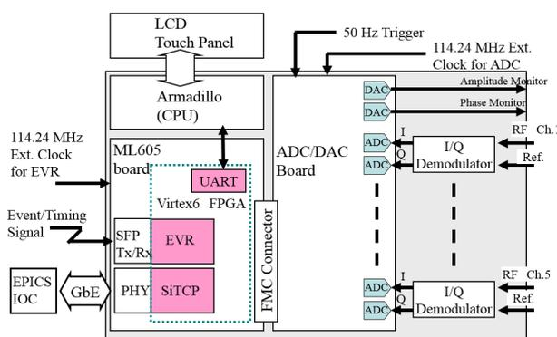
Figure 2: Block diagram of RF monitor unit.
