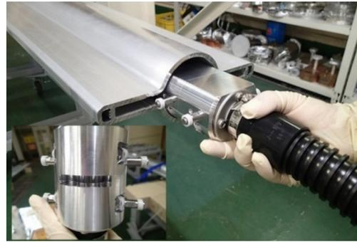
Figure 13: Special tool for collecting dust particles at the bottom of beam channel.
