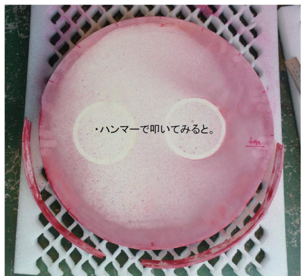
Figure 6: Broken RF window after checking cracked area (view from water-side).
