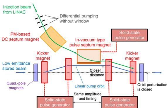
Figure 1: Schematic of the off-axis in-vacuum beam injection system. The kicker magnets and the pulse generators are also shown.
