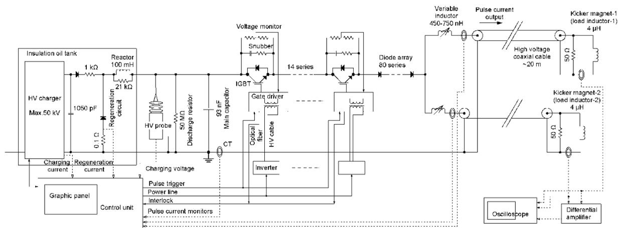
Figure 2: Block diagram for the pulse generator.
