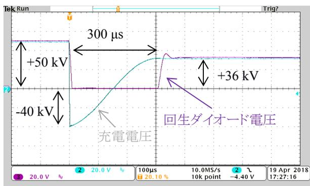
Figure 4: Waveform of the energy regeneration test.
