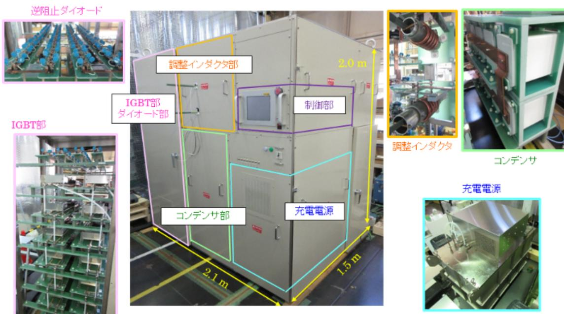
Figure 3: Photograph of the pulse generator.
