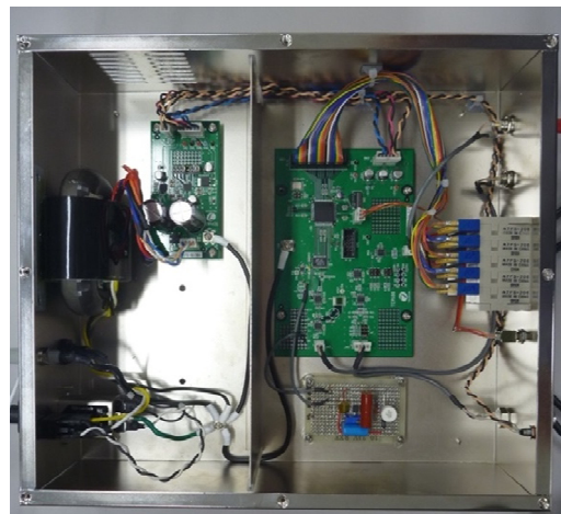
Figure 2: Inside of the developed offset amplifier. The left side is the power supply section, the right center is the low noise amplification circuit, the lower right is the reference voltage circuit.
