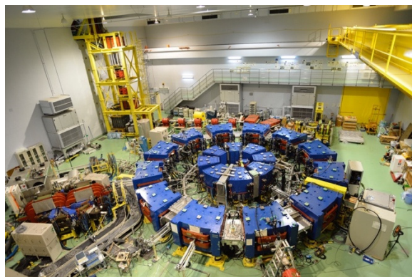
Figure 1: Photograph of main ring of 150 MeV FFAG accelerator at KURNS.
