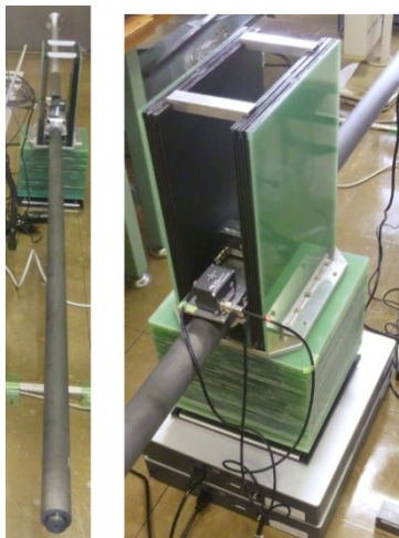
Figure 12: Set-up configuration of the newest type of vibration measurement system (2019 version).
