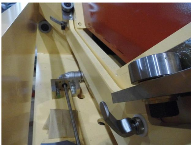
Figure 7: Stopper handles for cradle mechanism.
