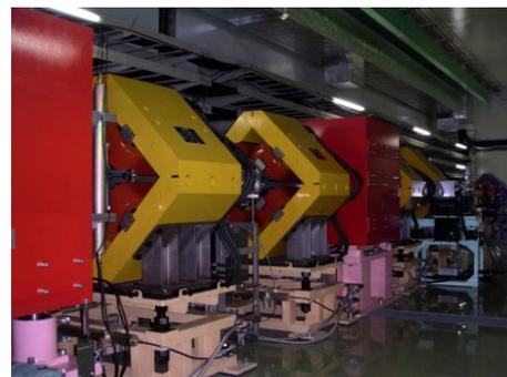
Figure 2: QSC family of quadrupole magnets.
