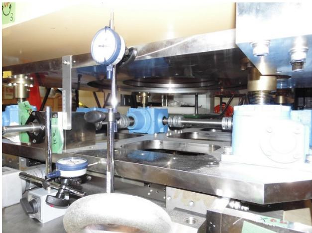
Figure 9: Independent stability monitoring for X and Z direction.
