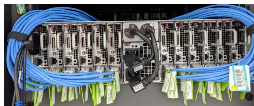
Figure 3: A photo of the SR cluster's front panel. A 3U chassis contains 24 servers.
