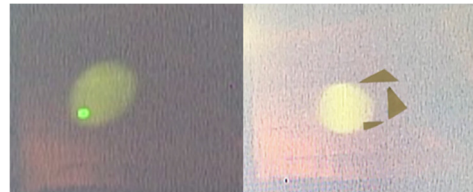
Figure 4: Effect of remanent magnetization of quadrupole magnets on the beam.
