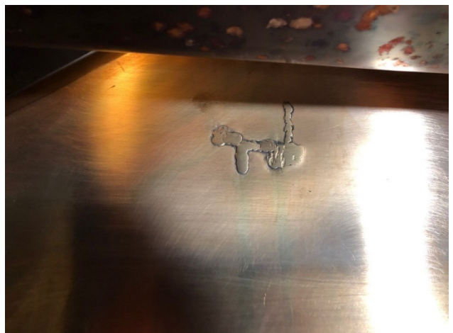
Figure 7: Resonator for RRC repaired in June 2020.
