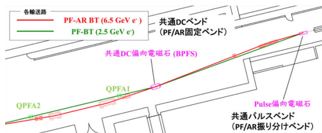
Figure 5: Electron beam transport lines for the PF-AR and the PF-Ring in Linac 3rd switch yard.
