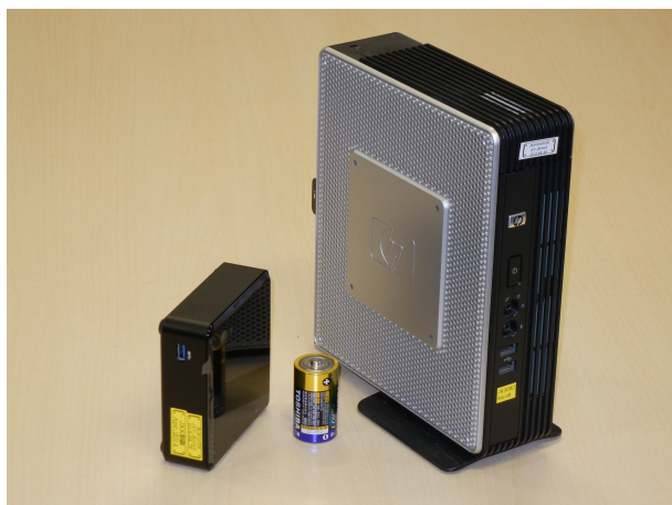
Figure 4: Intel NUC (left) and Thin-client (right).
