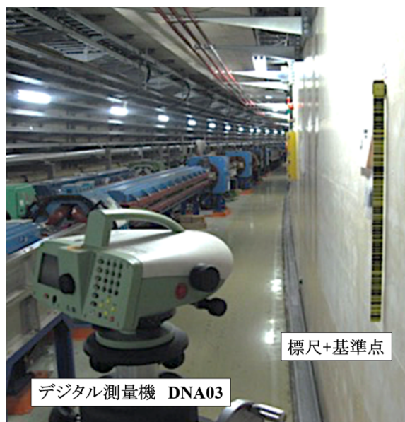
Figure 2: Surveying by DNA03.
