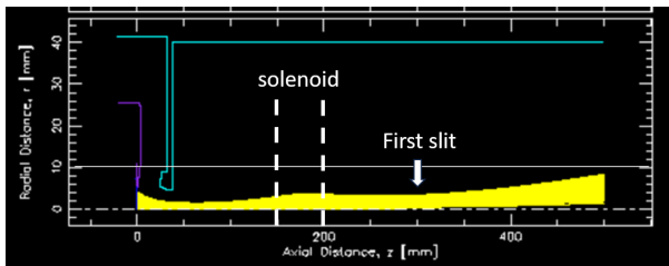
Figure 11: Electron beam trajectory after focusing.
