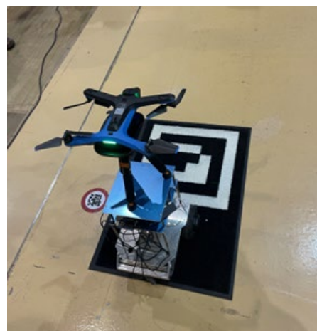
Figure 7: Drone landing base on transport robot.
