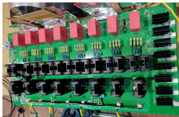
Figure 5: MARX Print-circuit board.
