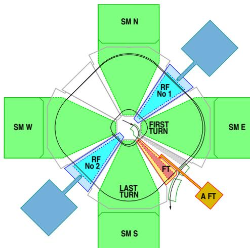
Figure 1: Layout of the RIKEN Ring Cyclotron with sector magnets (SM), main resonators (RF No 1 and 2) and flat-top system. The flat-top resonator is labeled with *FT*, and its amplifier system with *A FT*.
