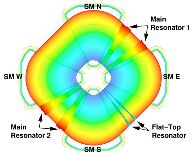
Figure 5: Visualization of the ion trajectory in the RRC with *MayaVi*. The coloring of the trajectory corresponds to the momentum of the particles and the set of arrows indicates the energy kick at the gap-crossings.
