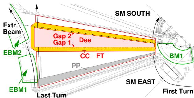
Figure 3: Top view on proposed valley box with flat-top resonator: phase probes (PP), capacitive coupler (CC), fine tuner (FT), injection-, extraction bending magnets (BM1, EBM1, EBM2) and sector magnets (SM).
