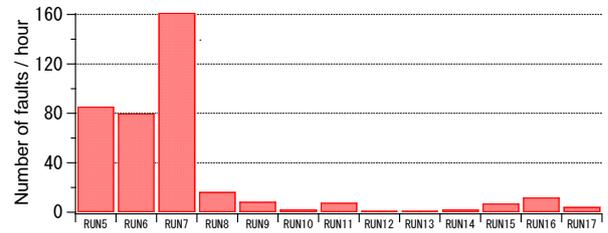
Figure 3: The rate of RF faults detected by LLRF fast interlock system
