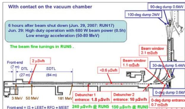
Figure 4: Residual radiation level after run 17.
