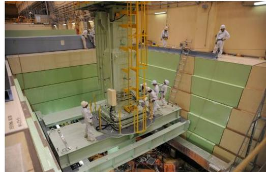
Fig. 3. *Transfer Cask* on the beam line over the muon target.
