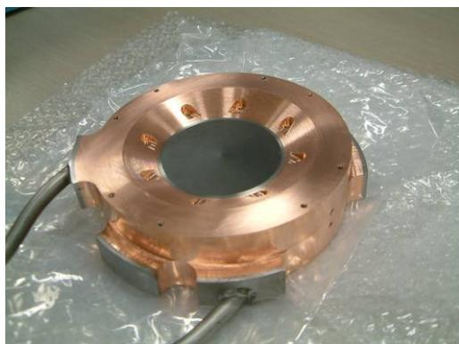
Fig. 1. Picture of the fabricated muon target.
