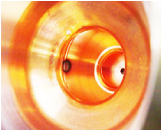
Figure 2: Picture of inner surface of the RF gun cavity after the first RF processing.
