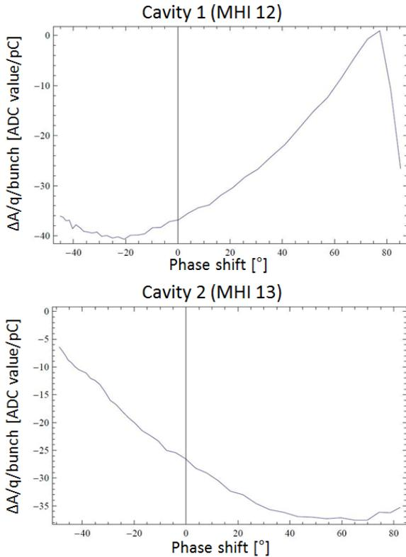
Figure 8: Beam induced amplitude  $\Delta A$ /charge per bunch versus RF phase shift for cavity 1 (top) and cavity 2 (bottom). The drop at cavity 1 above  $77^\circ$  of RF phase shift originates from effects of far off-crest beam operation.
