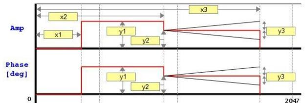
Figure 1: RF pulse shape properties for amplitude (top) and phase (bottom).
